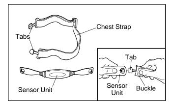
Next, wrap the chest pulse sensor around your chest and attach the other end of the chest strap to the sensor unit. Adjust the length of the chest strap, if necessary. The chest pulse sensor units expected the chest pulse sensor units are chest pulse sensor units.
